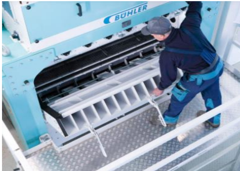
Figure.6 cleaning and maintaining oilseed cleaning machine
